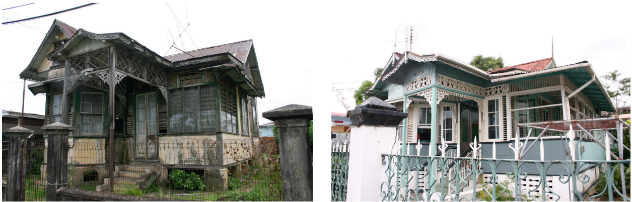
fig. 10. Caribbean townhouses may stand on posts as seen in the neglected “Sea Villa” house (left) (some gingerbread houses were given proper names by owners); or sit on hollow plinths aerated by wooden openwork, metallic or “fancy brick” ventilation panels as seen here on the “Rose Ville” house (right), Woodbrook, Port-of-Spain, Trinidad. Photographs by author.
